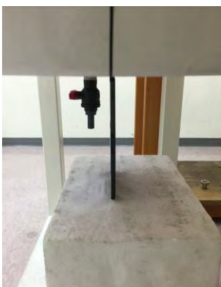
Fig.5 EUT Bottom side to flat phantom
