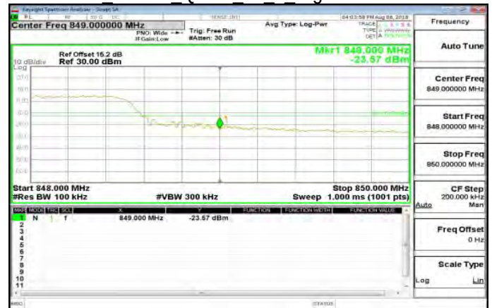
Band12 1 4MHz QPSK 1 0 LowCH23017-699.7
