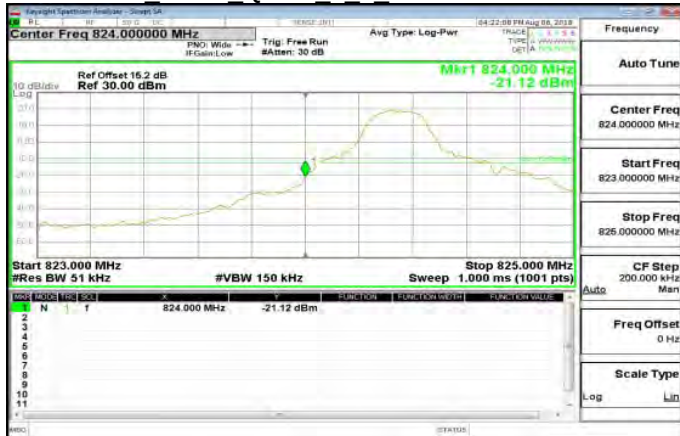
Band5 5MHz QPSK 1 0 LowCH20425-826.5
