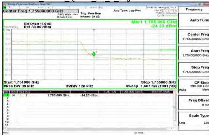
Band4 5MHz QPSK 1 0 LowCH19975-1712.5
