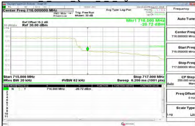
Band12 3MHz QPSK 1 0 LowCH23025-700.5
