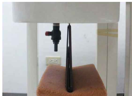
Fig.5 EUT (TB mode) Bottom side to flat phantom
