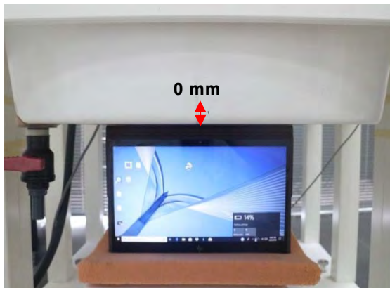
Fig.4 EUT Top side to flat phantom
