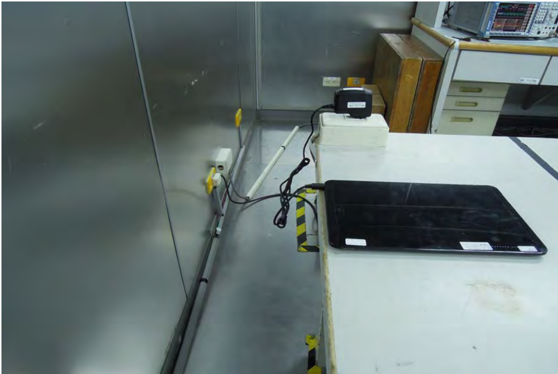
AC Power-line Conducted Emission Set up Photo
