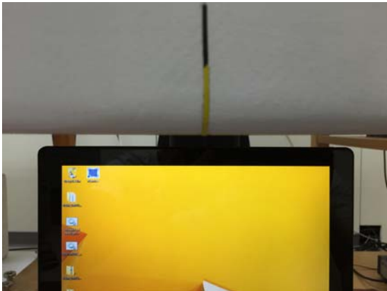
Fig.6 EUT Top side (12mm) to flat phantom
