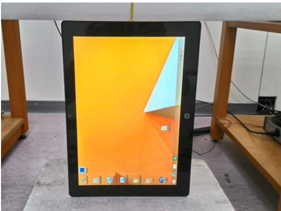
Fig.7 EUT Right side to flat phantom
