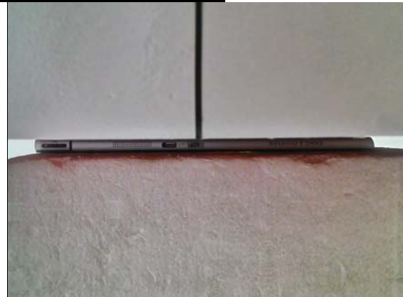
Fig.3 EUT Back side to flat phantom
