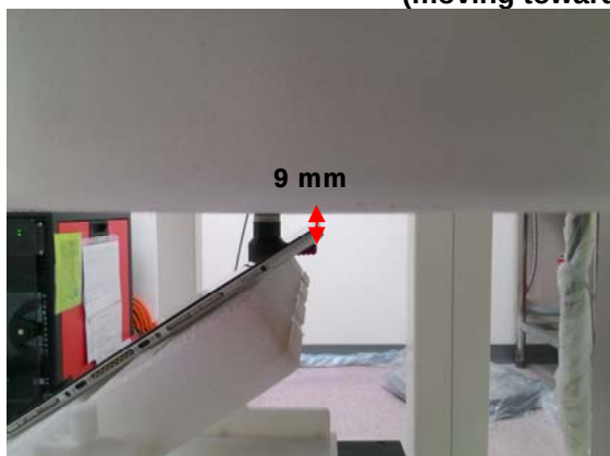
Fig.11 Tilt angle testing for right side (+45 degree) (moving toward/away from the phantom)
