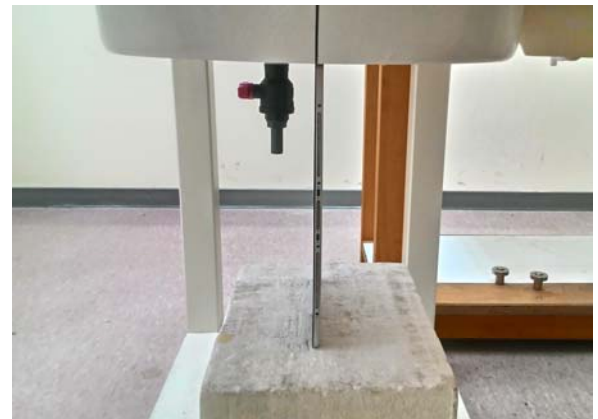
Fig.7 EUT Right side to flat phantom
