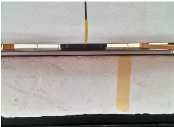
Fig.4 EUT Back side (12mm) to flat phantom
