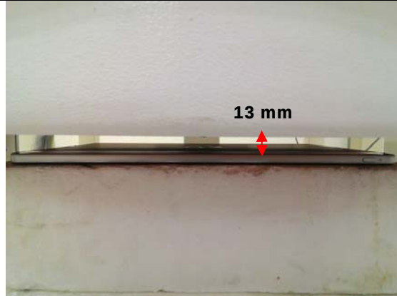
Fig.9 Trigger distance for backside (moving toward/away from the phantom)
