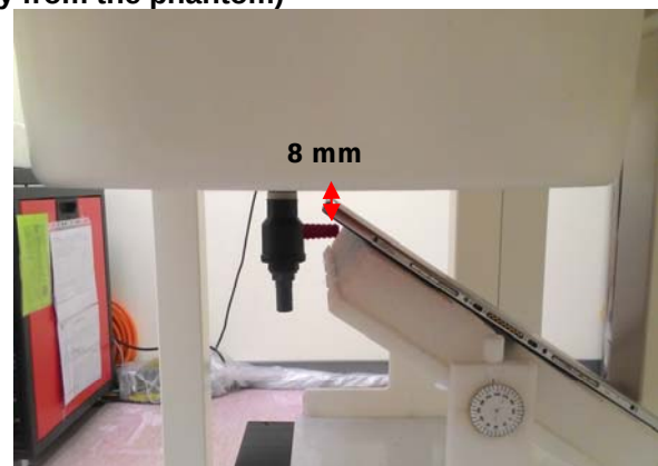
Fig.11 Tilt angle testing for right side (+45 degree) (moving toward/away from the phantom)
