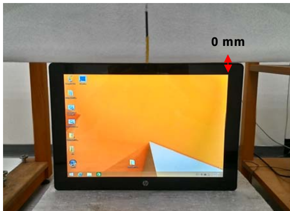
Fig.5 EUT Top side to flat phantom
