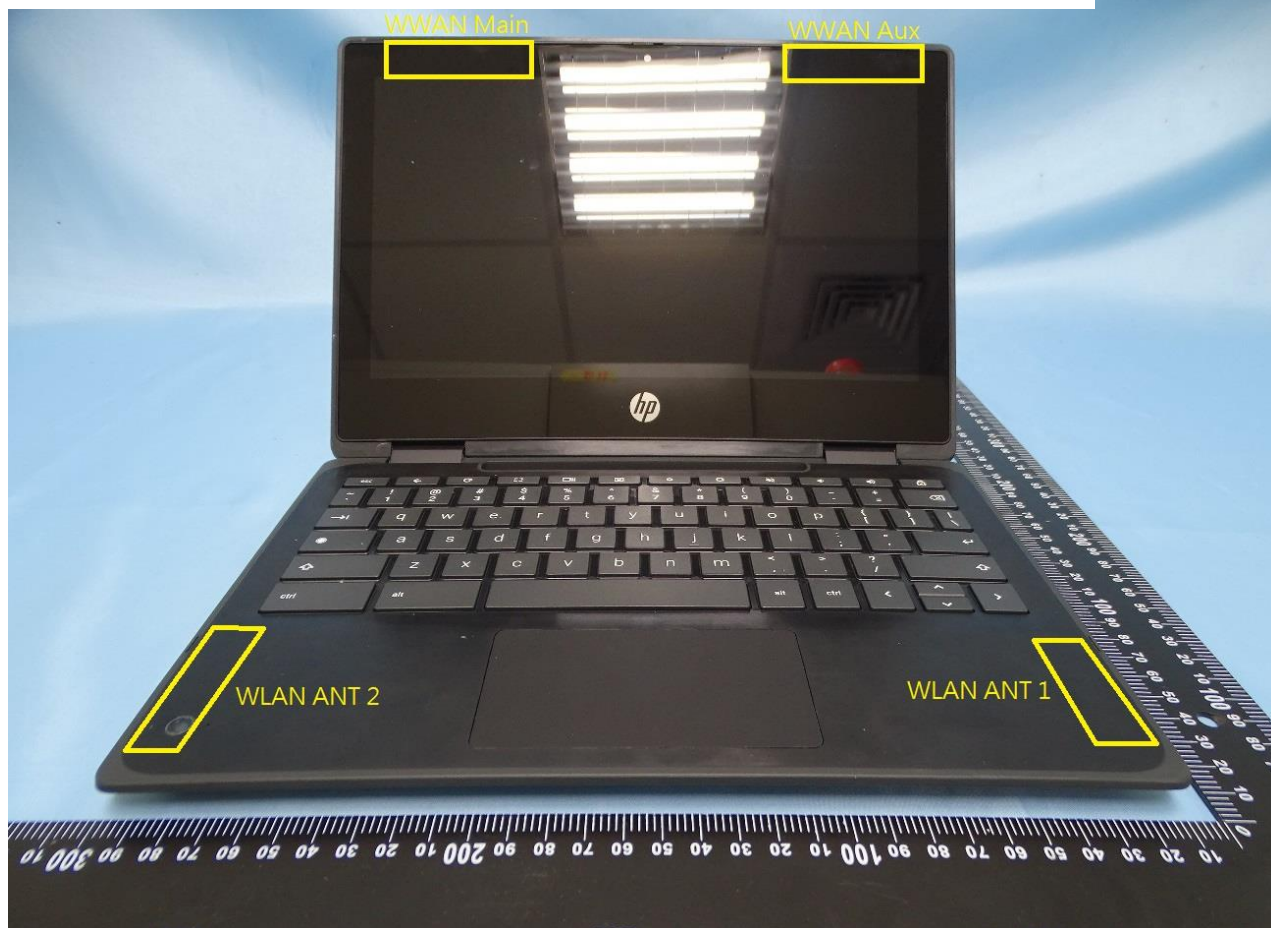
Vendor 1 Antenna and Vendor 2 Antenna with WWAN Module and WLAN Module
