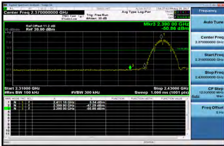
802.11b: Band Edges Test Data CH-High
