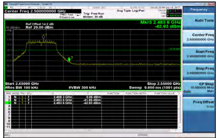
802.11n_HT20: Band Edges Test Data CH-13
