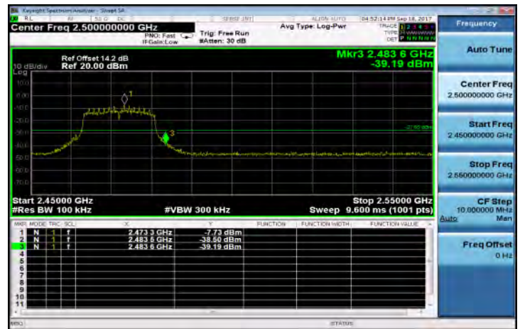
802.11n_HT20: Band Edges Test Data CH-13
