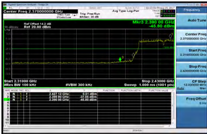
802.11n_HT40: Band Edges Test Data CH-High
