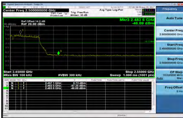
802.11n_HT40: Band Edges Test Data CH-High
