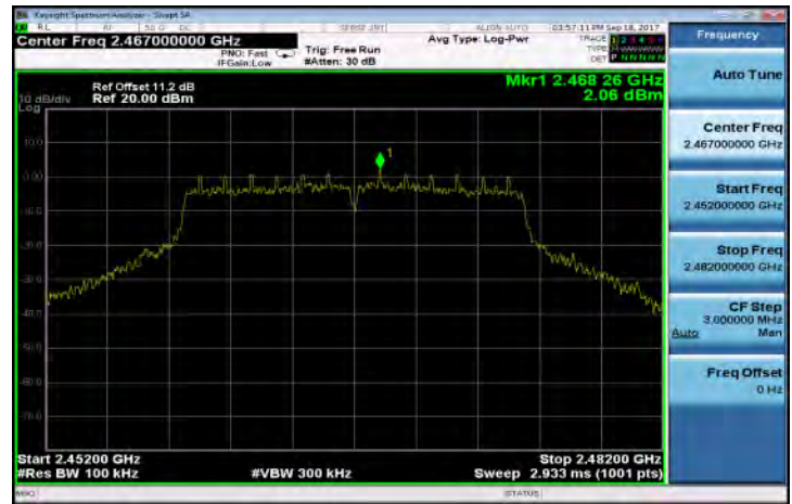
802.11g PSD for Bandedge Limit(CH-13)
