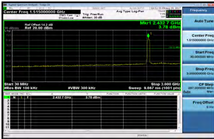
802.11n_HT40: Spurious Emission Test Data CH-Mid
