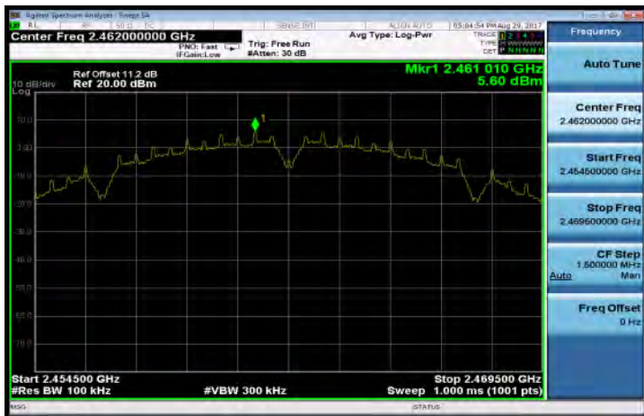
802.11b PSD for Bandedge Limit(CH-High)
