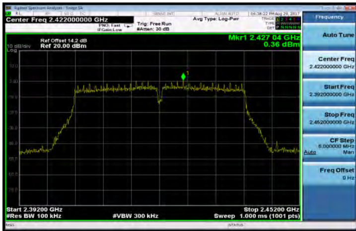
802.11n_HT40 PSD for Bandedge Limit(CH-High)
