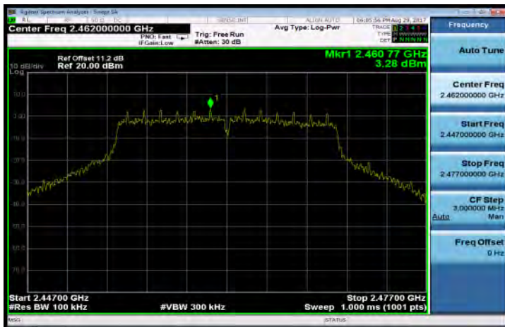
802.11g PSD for Bandedge Limit(CH-High)
