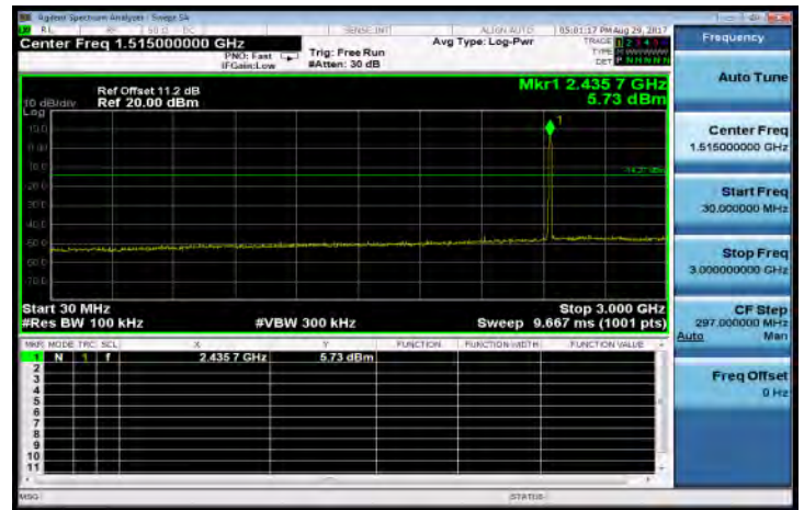
802.11b: Spurious Emission Test Data CH-Mid
