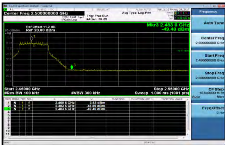
802.11g: Band Edges Test Data CH-High
