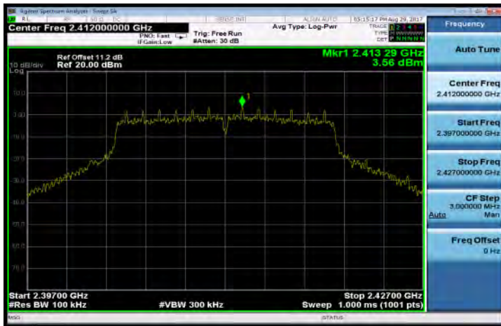
802.11g PSD for Bandedge Limit(CH-High)
