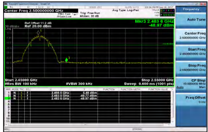
802.11b: Band Edges Test Data CH-13
