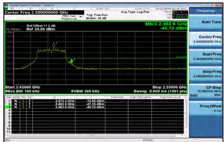
802.11g: Band Edges Test Data CH-13
