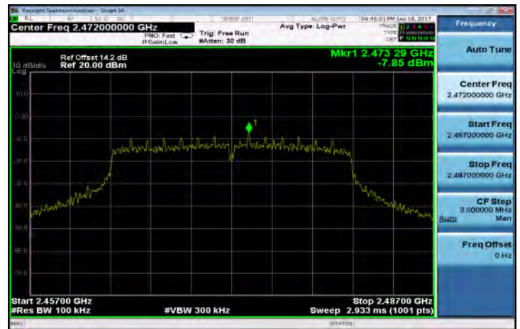
802.11n_HT20 PSD for Bandedge Limit(CH-13)
