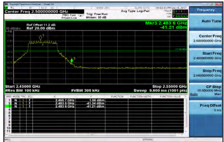
802.11g: Band Edges Test Data CH-13
