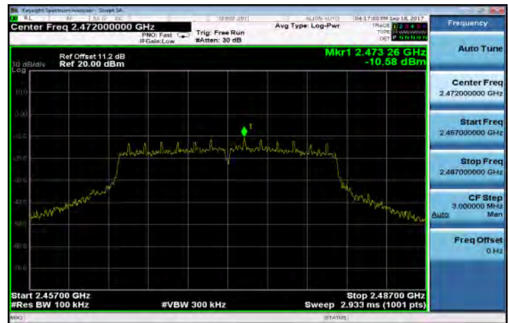
802.11g PSD for Bandedge Limit(CH-13)
