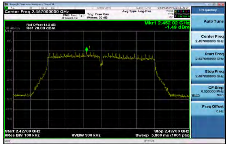
802.11n_HT40 PSD for Bandedge Limit(CH-11)
