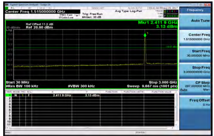
802.11g: Spurious Emission Test Data CH-Low
