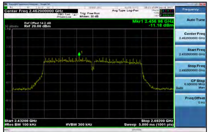
802.11n_HT40 PSD for Bandedge Limit(CH-11)
