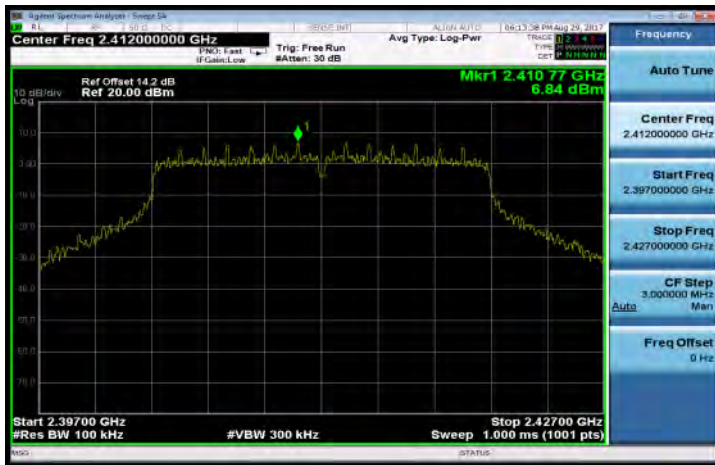
802.11n_HT20 PSD for Bandedge Limit(CH-High)
