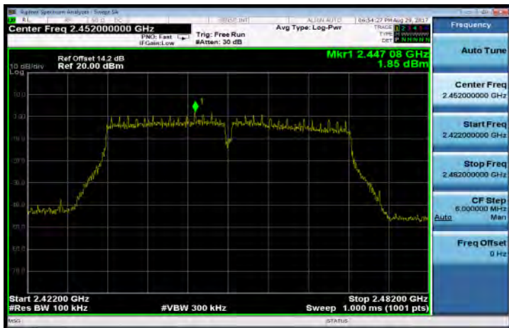
802.11n_HT40 PSD for Bandedge Limit(CH-High)
