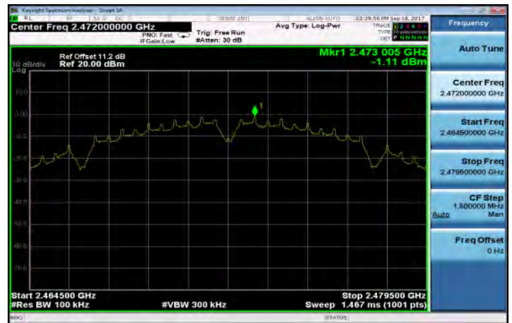
802.11b PSD for Bandedge Limit(CH-13)
