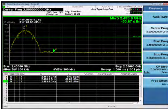
802.11b: Band Edges Test Data CH-High
