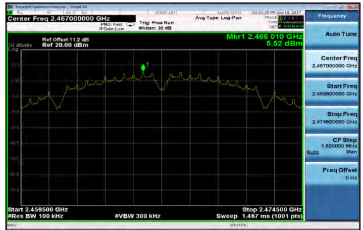
802.11b PSD for Bandedge Limit(CH-13)
