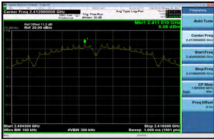
802.11b PSD for Bandedge Limit(CH-High)
