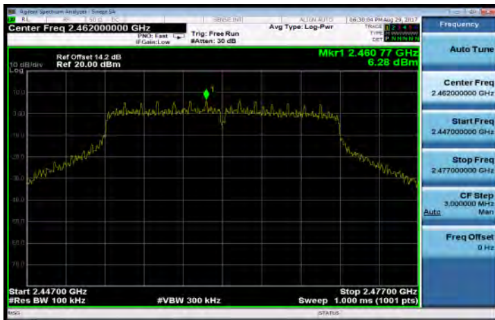
802.11n_HT20 PSD for Bandedge Limit(CH-High)
