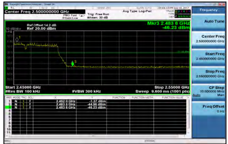
802.11n_HT40: Band Edges Test Data CH-11
