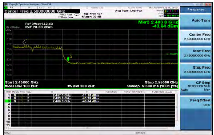
802.11n_HT40: Band Edges Test Data CH-11
