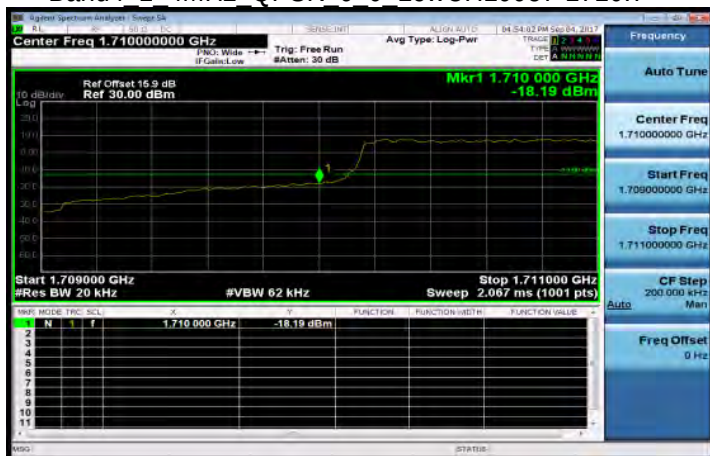
Band4 1 4MHz QPSK 6 0 LowCH19957-1710.7
