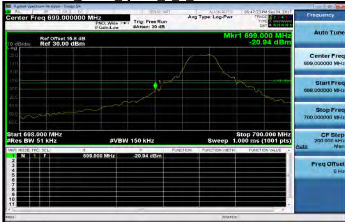
Band12 5MHz QPSK 1 0 LowCH23035-701.5
