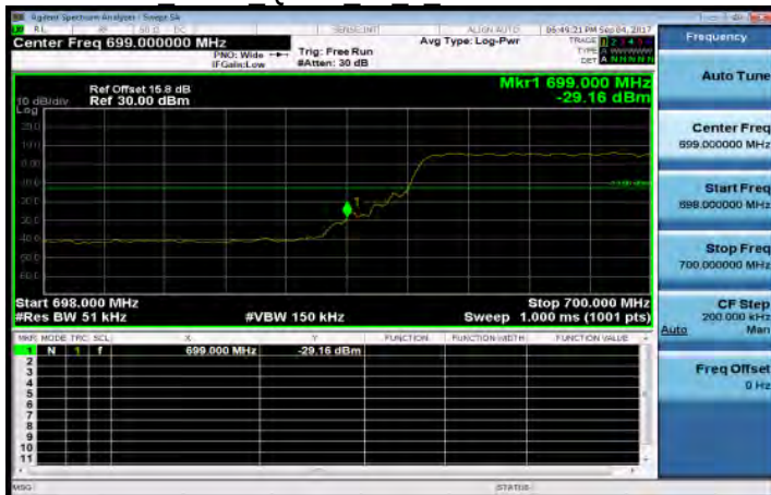
Band12 5MHz QPSK 25 0 LowCH23035-701.5
