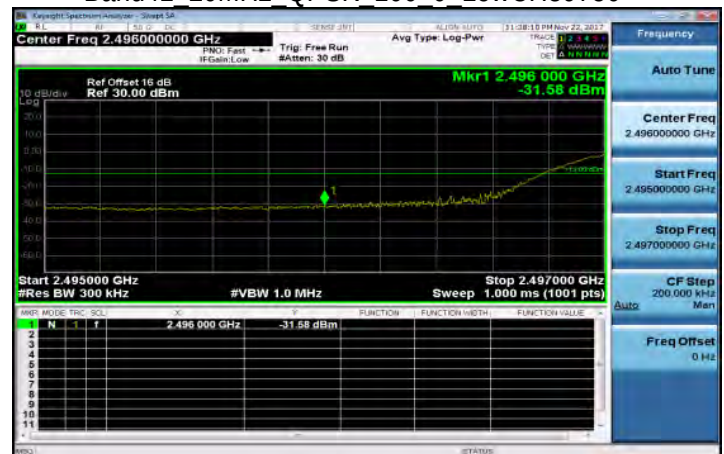
Band41 20MHz QPSK 100 0 LowCH39750
