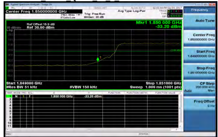
Band2 5MHz QPSK 25 0 LowCH18625-1852.5
