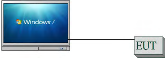
Fig. 2-1 Conducted (Antenna Port) Emission Configuration
