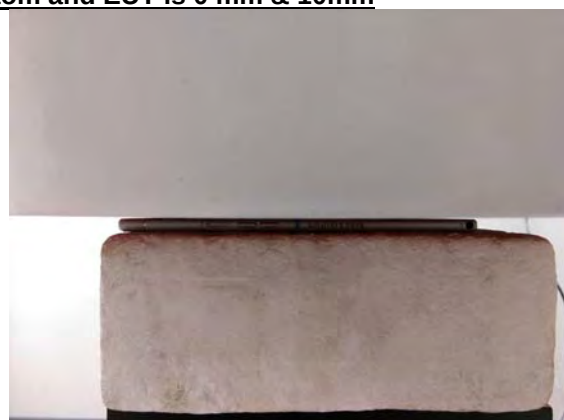
Fig.3 EUT Back side to flat phantom
