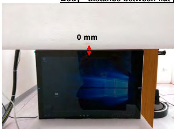
Fig.6 EUT Top side to flat phantom
