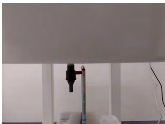
Fig.7 EUT Top side (10mm) to flat phantom
