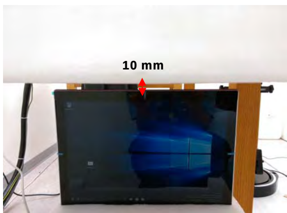
Fig.7 EUT Top side (10mm) to flat phantom
