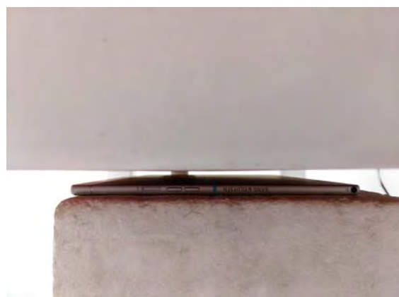
Fig.4 EUT Back side (10mm) to flat phantom
