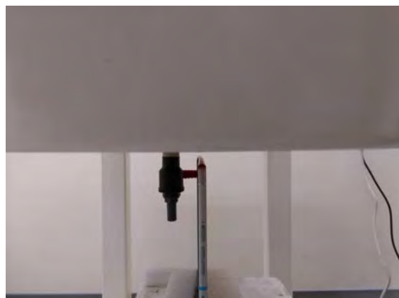
Fig.7 EUT Top side (10mm) to flat phantom
