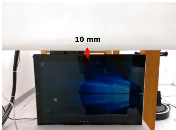
Fig.7 EUT Top side (10mm) to flat phantom
