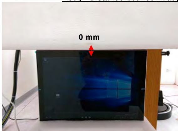
Fig.6 EUT Top side to flat phantom
