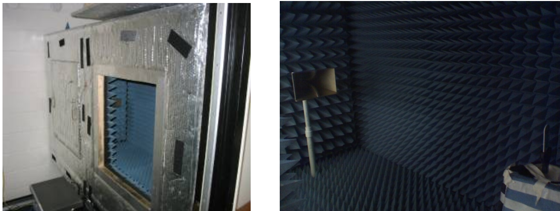
Figure 23. The anechoic chamber (left) used for testing antennas eliminating secondary reflections, and the interior of the anechoic chamber (right) containing the horn antenna on the left and the tested antenna on the right
