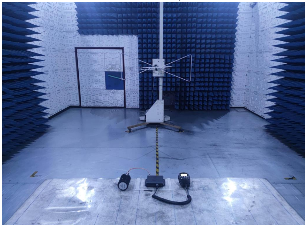
Radiated Emission Test Setup-Above 30MHz
