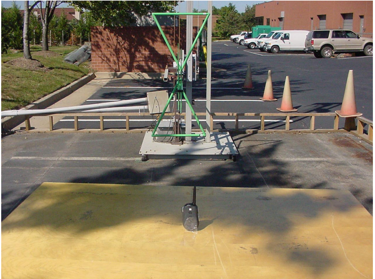
PHOTOGRAPH 1: RADIATED TEST CONFIGURATION (REAR VIEW)
