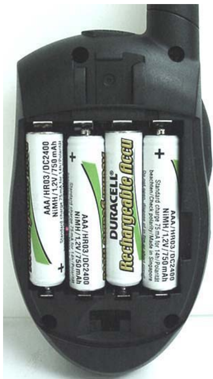
DUT with NiMH AAA Batteries
