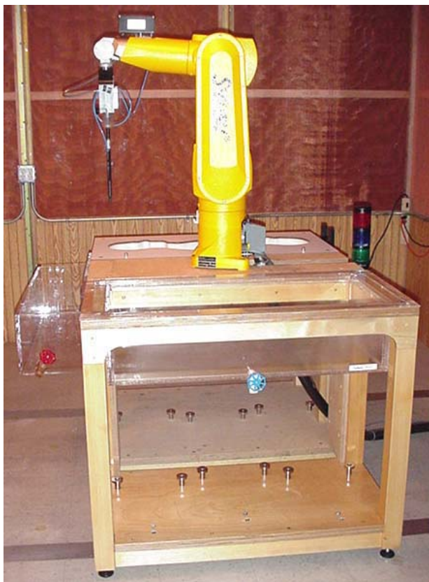
DASY4 SAR Measurement System with validation phantom
