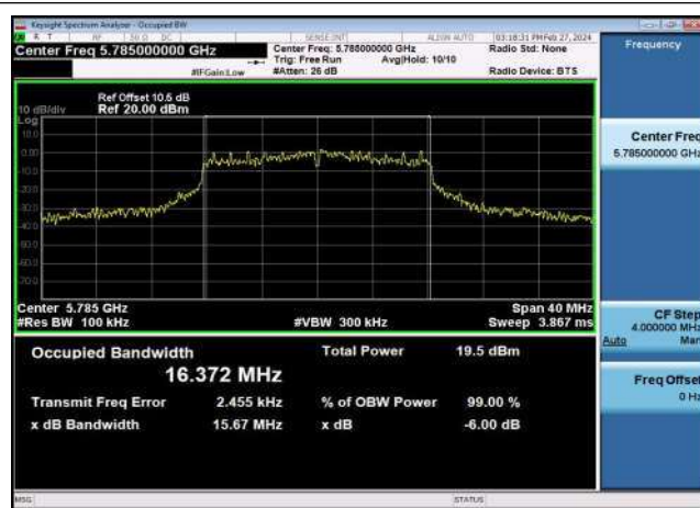
U-NII-3 6dB Bandwidth-802.11ac(20MHz) ,5745MHz,Ant1
