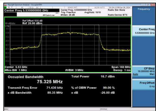
U-NII-3 99% & 26dB Bandwidth-802.11n(20MHz),5785MHz,Ant1
