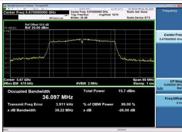
U-NII-3 99% & 26dB Bandwidth-802.11n(20MHz),5745MHz,Ant1
