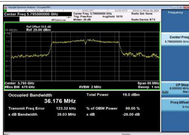
U-NII-3 99% & 26dB Bandwidth-802.11a(20MHz) ,5785MHz,Ant1
