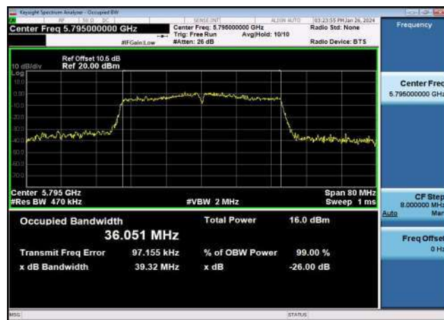
U-NII-3 99% & 26dB Bandwidth-802.11ac(40MHz) ,5795MHz,Ant1
