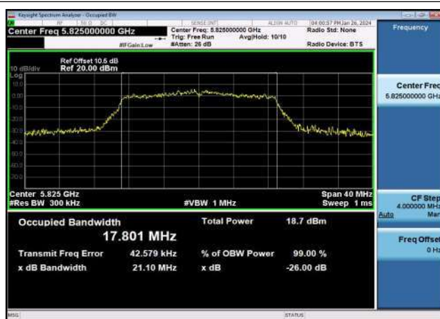
U-NII-3 99% & 26dB Bandwidth-802.11n(20MHz),5825MHz,Ant1
