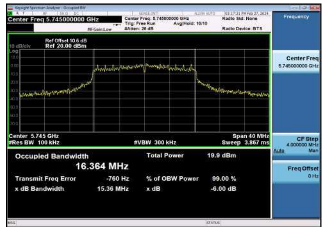
U-NII-3 6dB Bandwidth-802.11a(20MHz) ,5745MHz,Ant1
