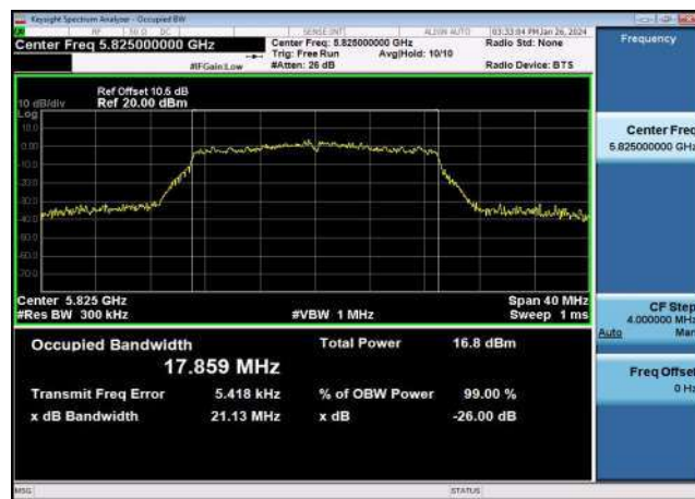
U-NII-3 99% & 26dB Bandwidth-802.11ac(40MHz) ,5795MHz,Ant1
