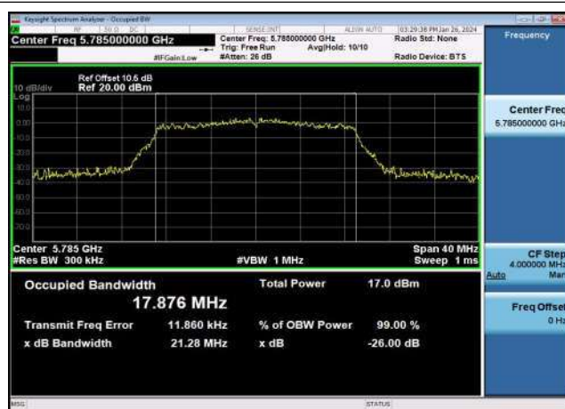
U-NII-3 99% & 26dB Bandwidth-802.11ac(20MHz) ,5785MHz,Ant1
