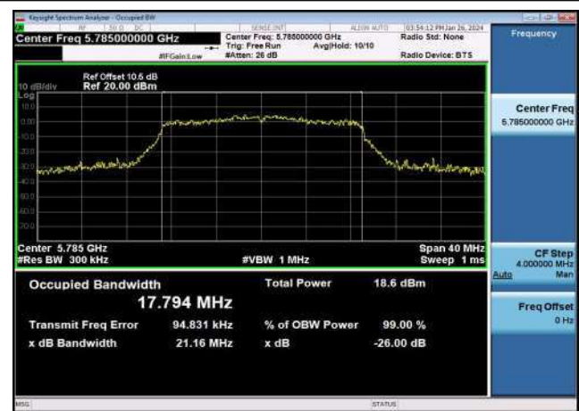
U-NII-3 99% & 26dB Bandwidth-802.11n(40MHz),5755MHz,Ant1
