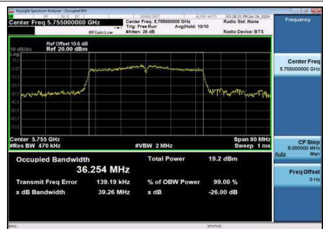
U-NII-3 99% & 26dB Bandwidth-802.11n(40MHz),5755MHz,Ant1
