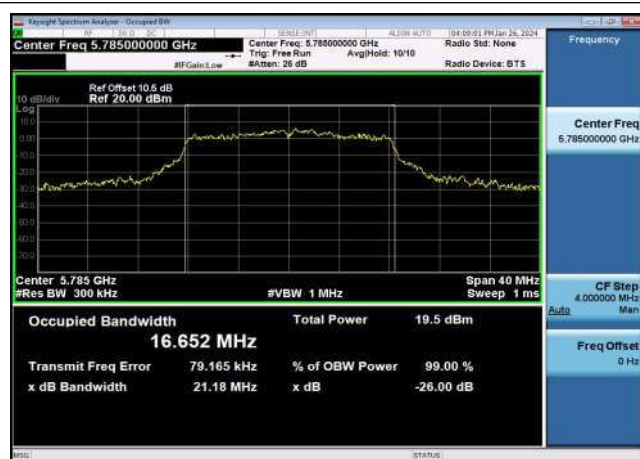
U-NII-3 99% & 26dB Bandwidth-802.11ac(20MHz) ,5745MHz,Ant1
