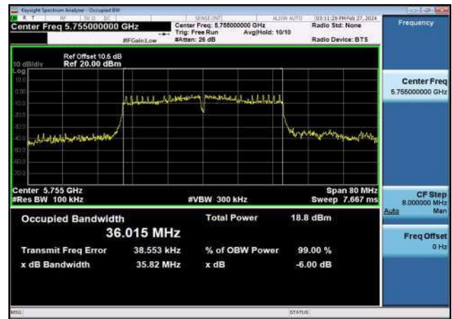
U-NII-3 6dB Bandwidth-802.11a(20MHz) ,5745MHz,Ant1
