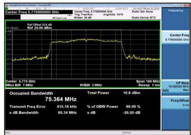
U-NII-3 99% & 26dB Bandwidth-802.11ac(80MHz) ,5775MHz,Ant1
