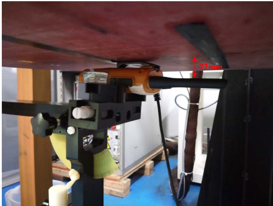
Body Back With Belt Clip and MIC Setup Photo (0mm)
