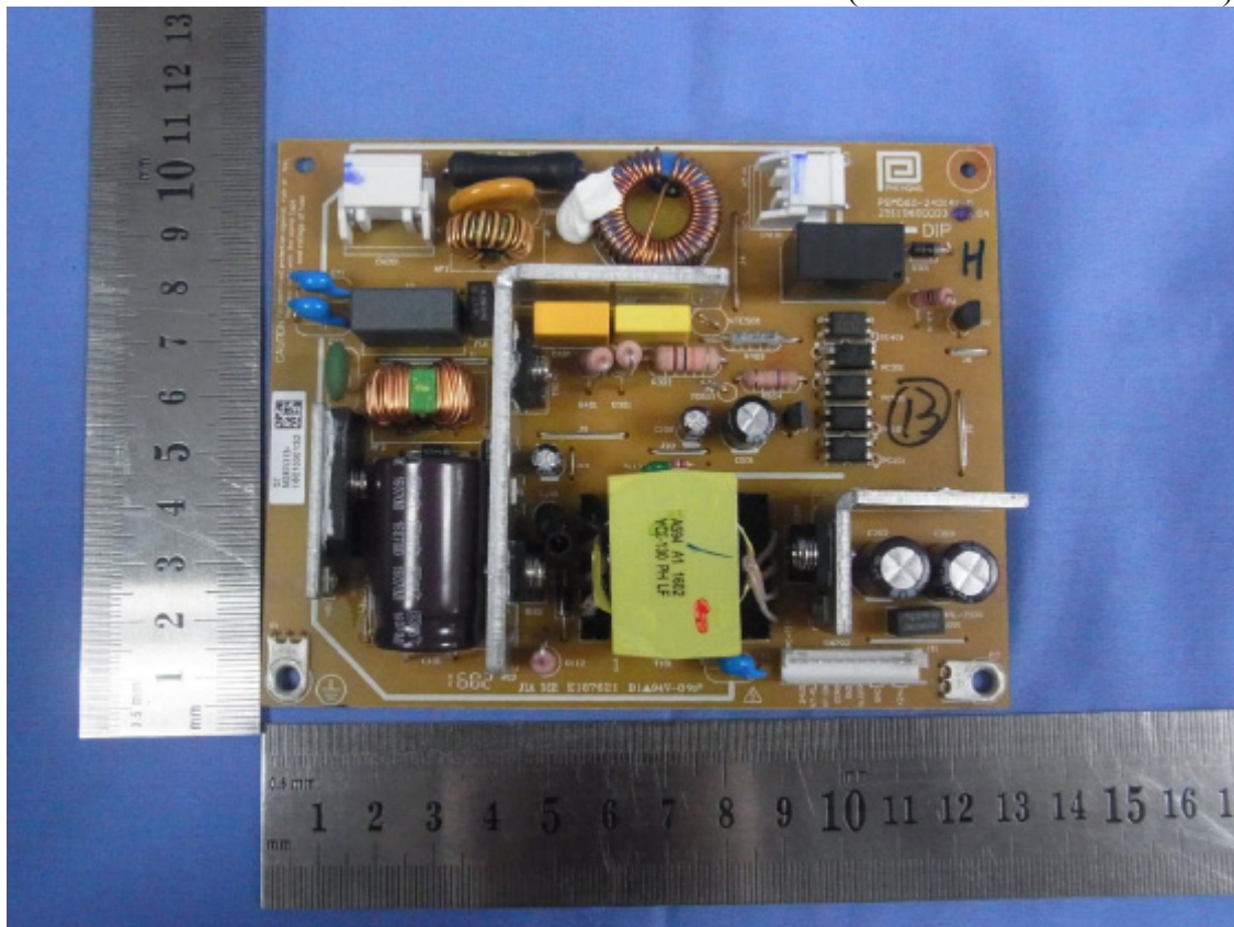
Figure 10 Internal View (Power Board/ Front View)
