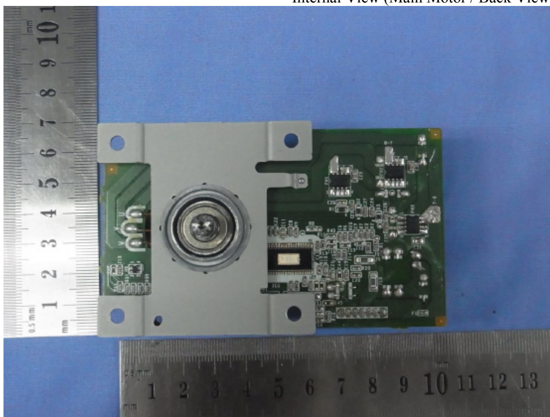
Figure 19 Internal View (Main Motor / Back View)
