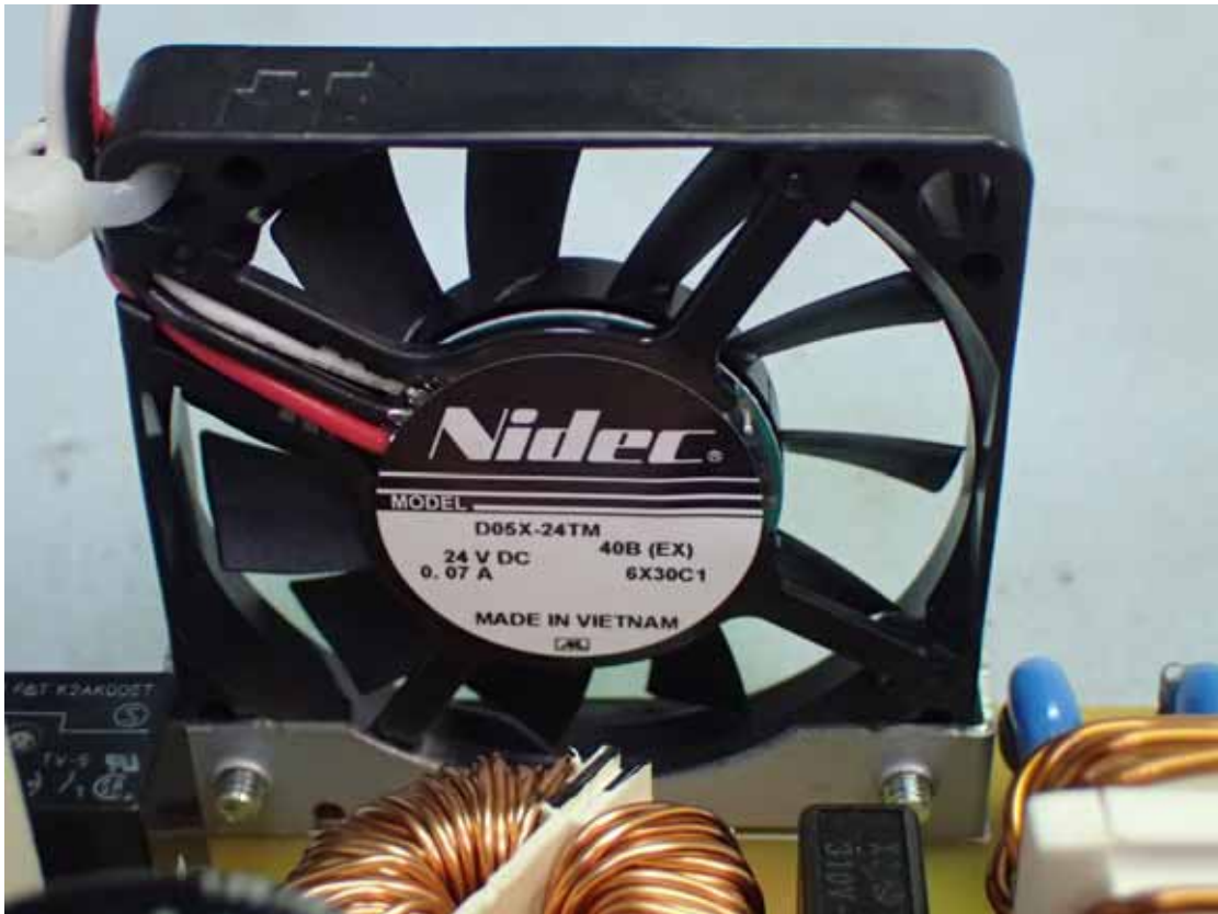
Figure 35 Internal View (DC Fan of Power Board)
