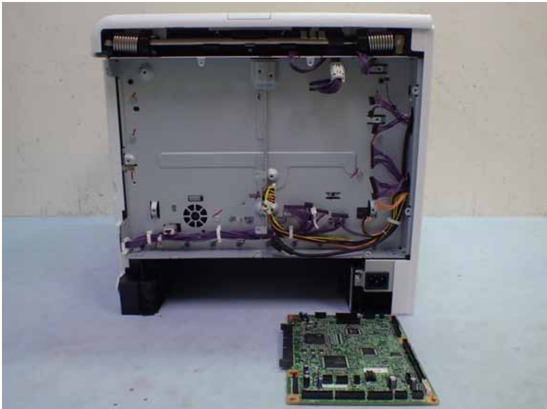
Figure 20 Internal View (Removed Main Board #1)
