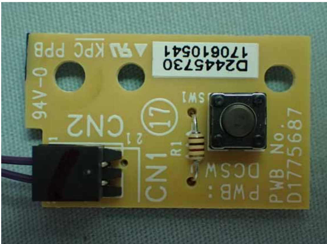
Figure 36 Internal View (SW Board, Front View)
