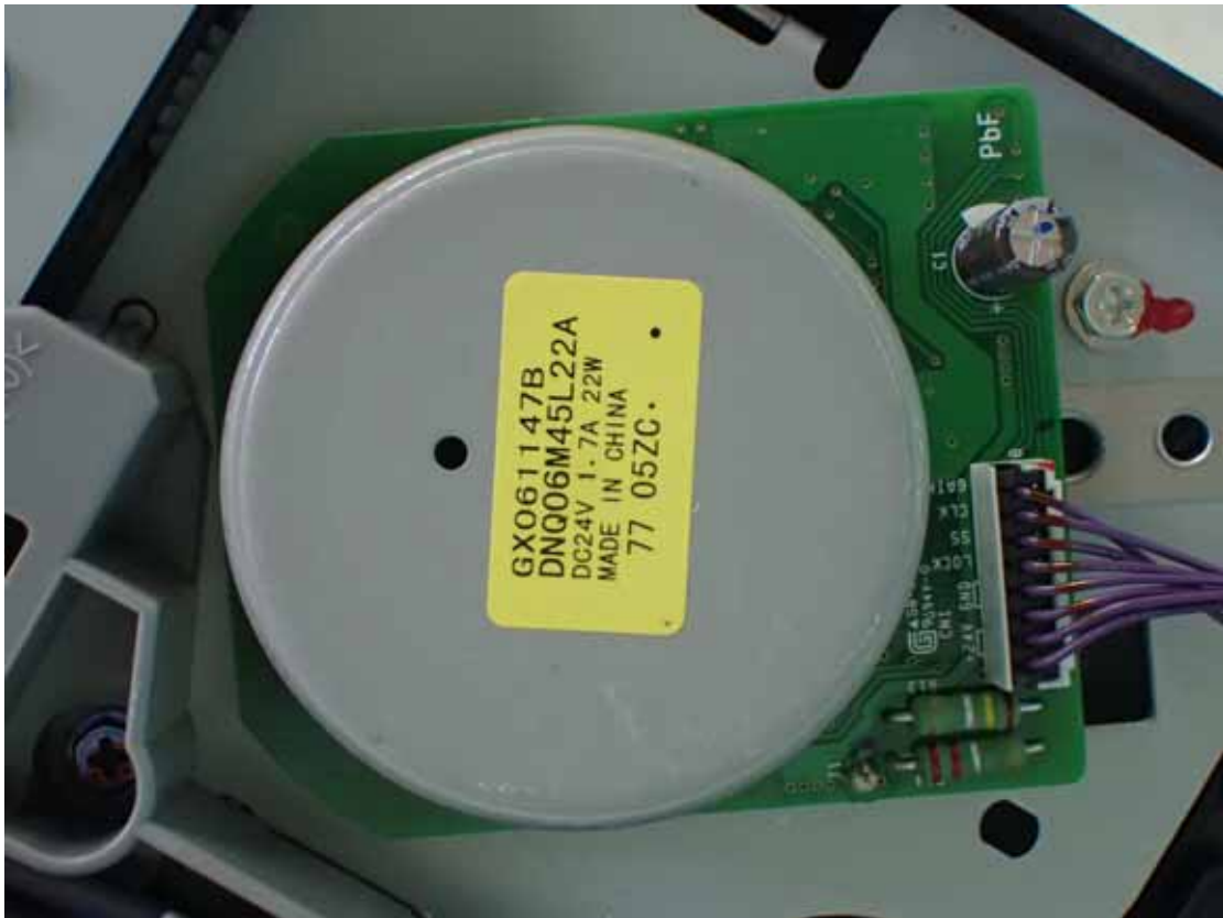
Figure 31 Internal View (Motor Board #3, Front View)
