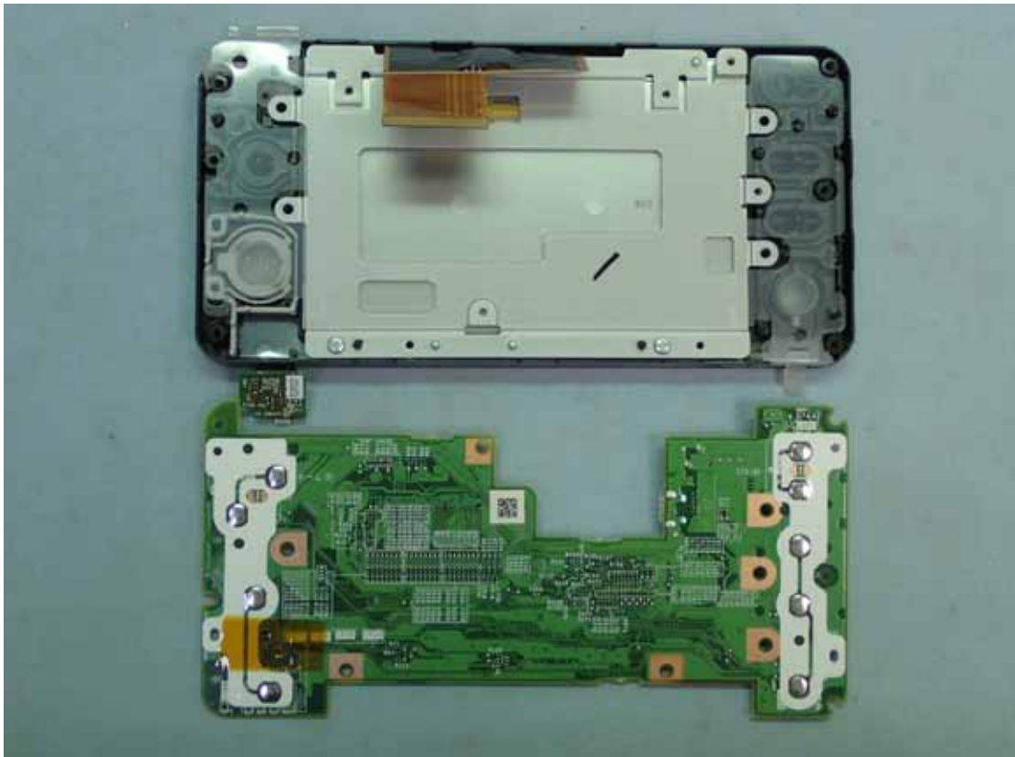
Figure 12 Internal View (Display Control Board, Back View)
