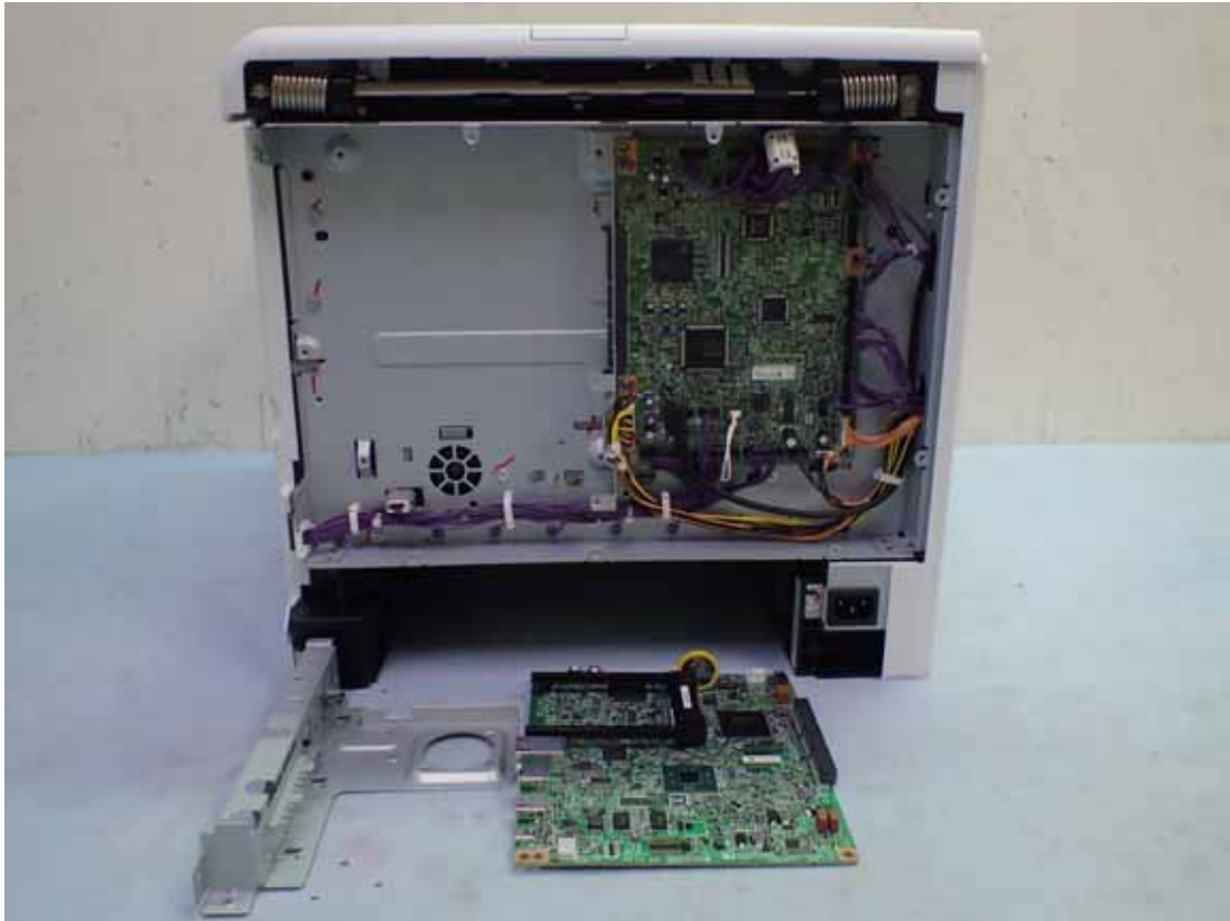
Figure 23 Internal View (Removed Main Board #2)
