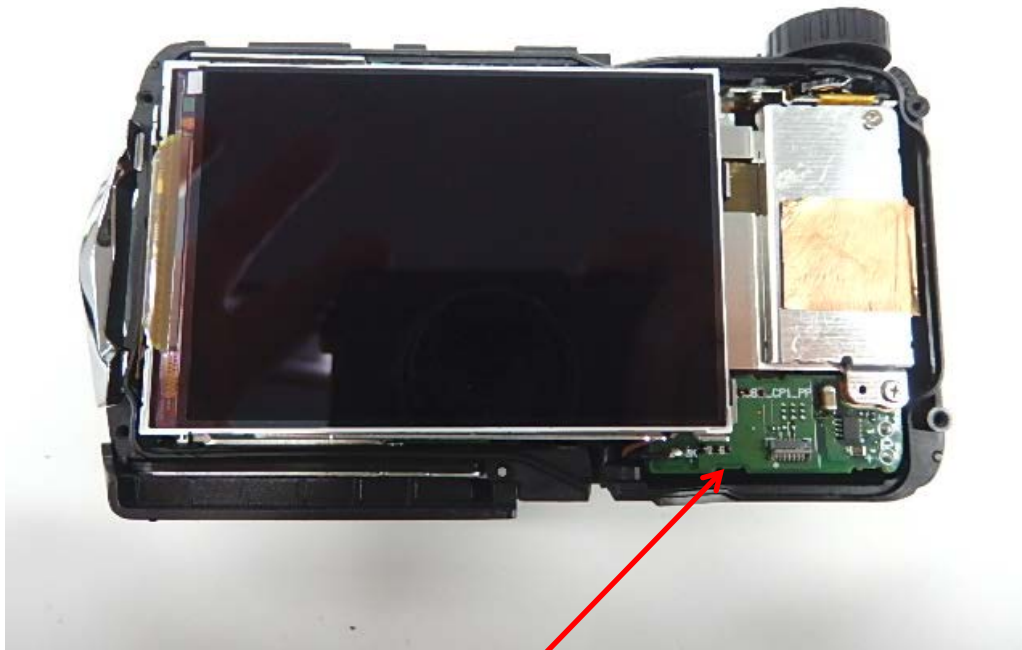
Location of CP1 Board (BT&WLAN)
