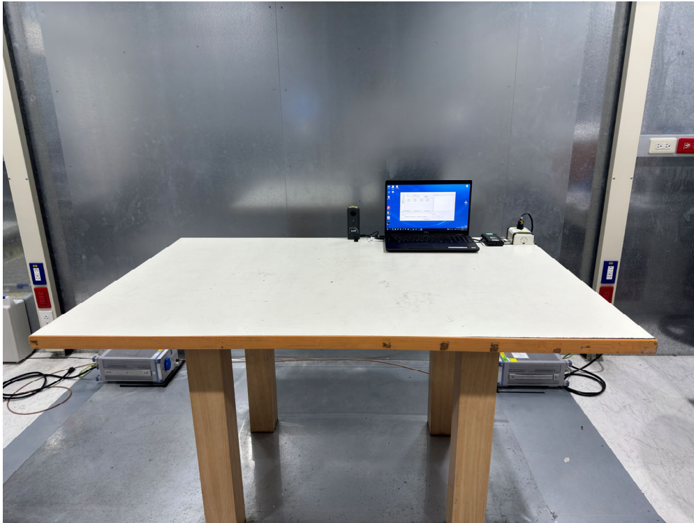
Back View of AC Power Line Conducted Emission Test
