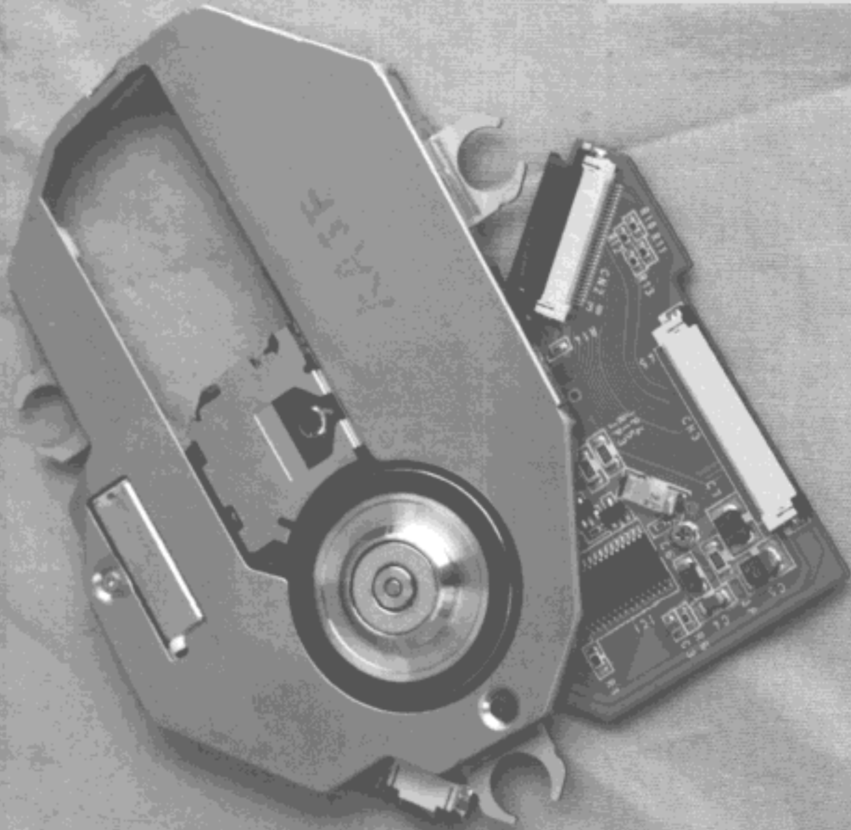
Fig.6 - Pickup Module (PCB Soldering Side) FCC ID:BBP7040A RICOH Co.,Ltd,
