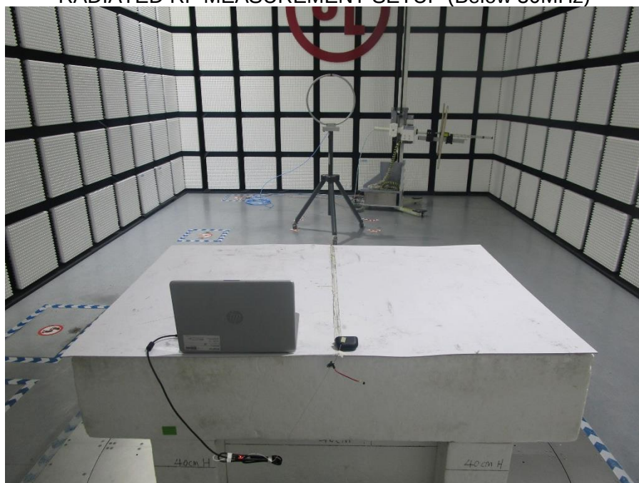
RADIATED RF MEASUREMENT SETUP (Below 30MHz)
