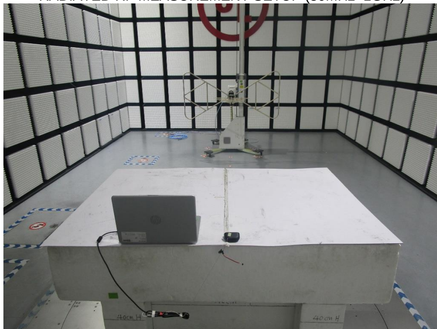
RADIATED RF MEASUREMENT SETUP (Below 30MHz)
