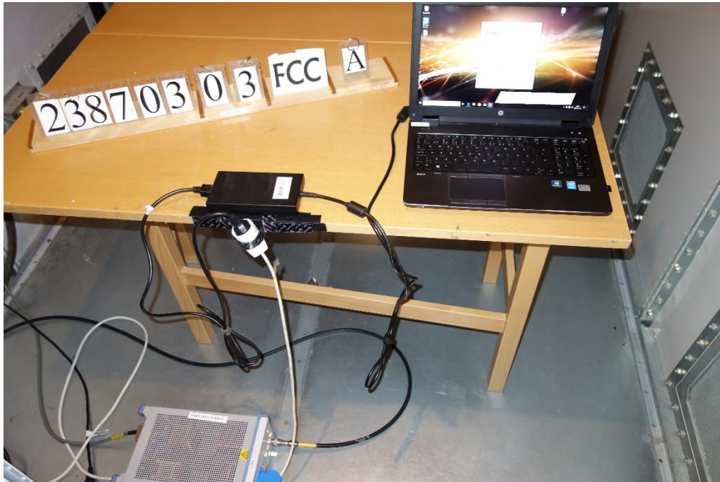
Test setup picture in Conducted Emission chamber
