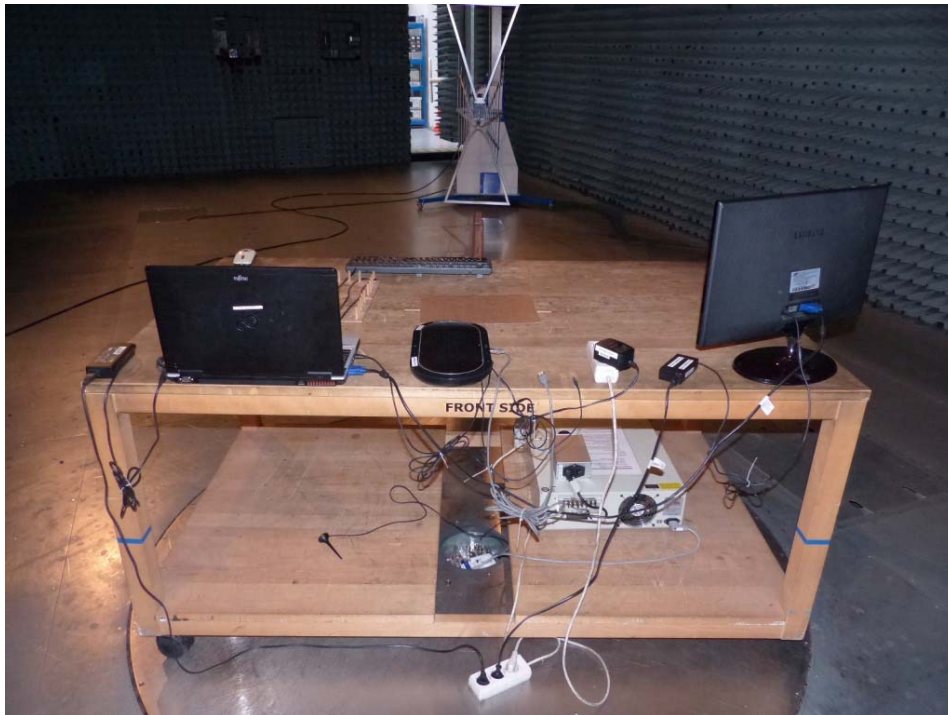
Photo 3: Test setup for radiated measurements in the range 30 – 1000 MHz, EUT supplied by AC/DC adapter, computer peripheral setup, used for unintentional radiator measurements.
