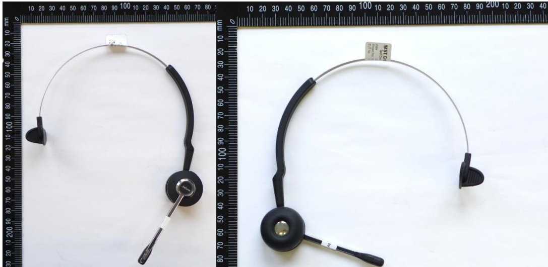
Pic. 3: View of the device under test with attached metal headband.
