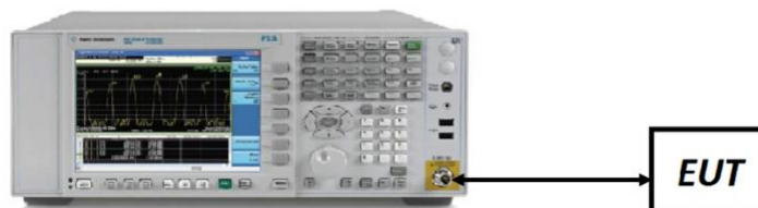
Figure 7-4. Test Instrument & Measurement Setup
