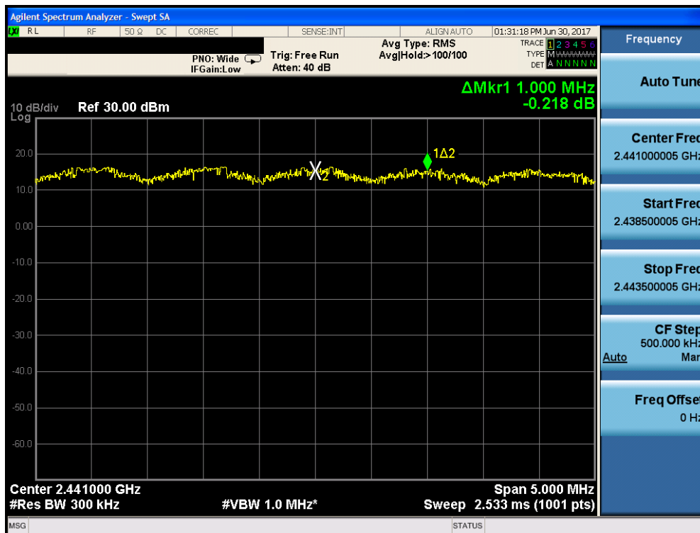
Plot 7-42. Channel Spacing Plot (Bluetooth, 8DPSK, ePA)
