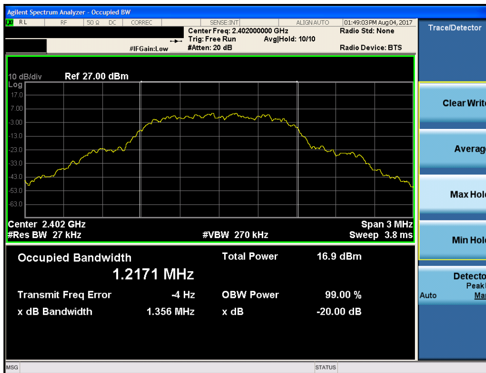
Plot 7-10. 20dB Bandwidth Plot (Bluetooth, 8DPSK, iPA – Ch. 0)
