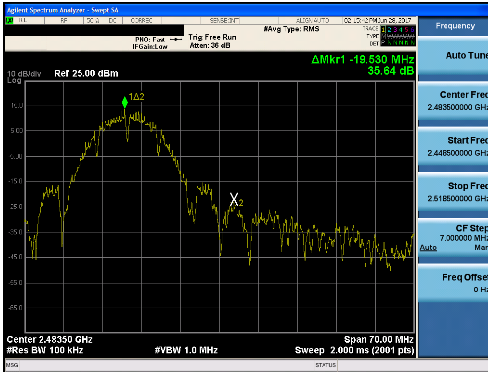
Plot 7-21. Band Edge Plot (802.11b – Ch. 12)
