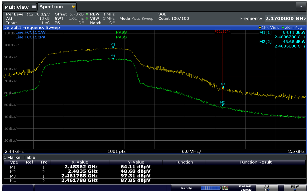
Plot 7-45. Radiated Restricted Upper Band Edge Measurement (Average & Peak)
