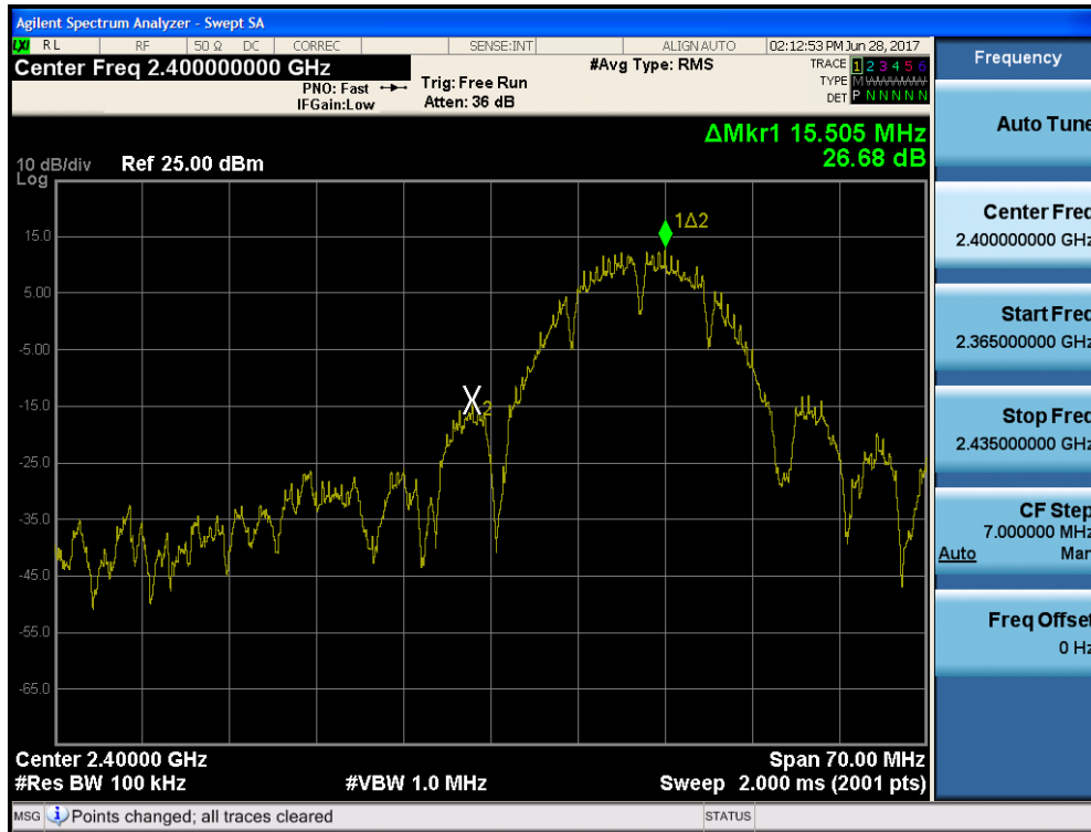
Plot 7-19. Band Edge Plot (802.11b – Ch. 1)
