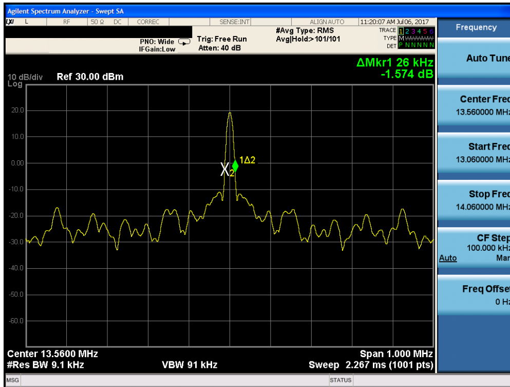
Figure 7-3. 20dB Bandwidth Plot (CE B 848kbps)
