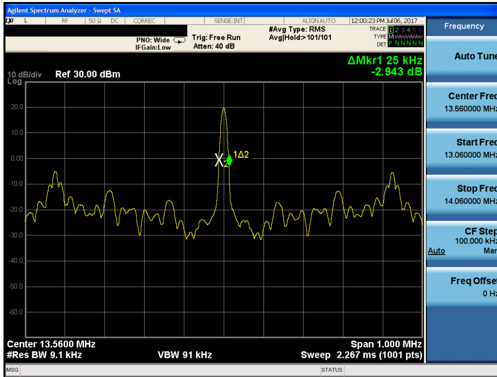
Figure 7-4. 20dB Bandwidth Plot (CE F 424kbps)
