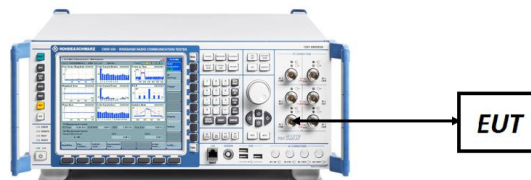
Figure 7-5. ERP/EIRP Measurement Setup
