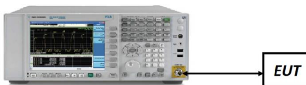
Figure 7-7. Test Instrument & Measurement Setup
