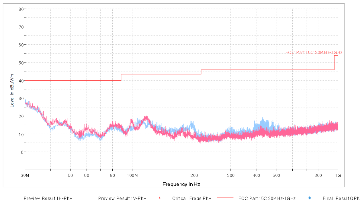
Plot 7-74. Radiated Spurious Plot below 1GHz (GFSK ePA, Pol. H & V)
