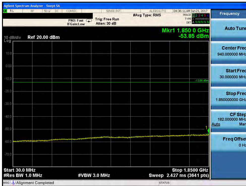
Plot 7-95. Conducted Spurious Plot (Band 2/25 – 1.4MHz QPSK – RB Size 1, RB Offset 0 – High Channel)
