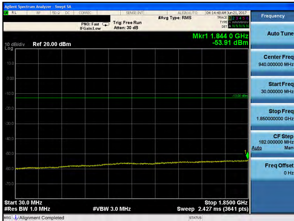
Plot 7-92. Conducted Spurious Plot (Band 2/25 – 1.4MHz QPSK – RB Size 1, RB Offset 0 – Mid Channel)
