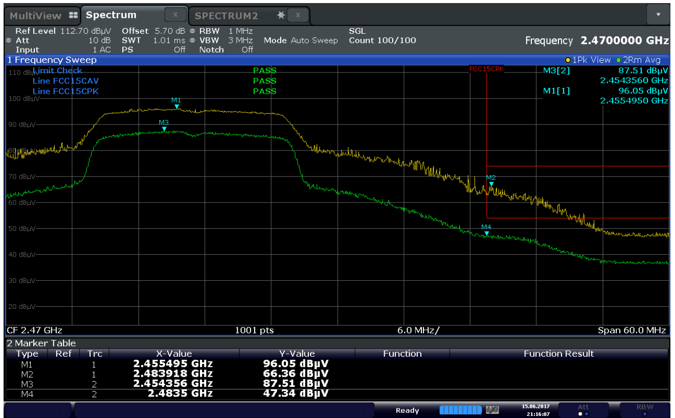
Plot 7-46. Radiated Restricted Upper Band Edge Measurement (Average & Peak)
