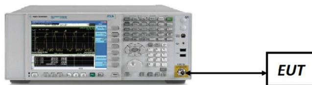
Figure 7-5. Test Instrument & Measurement Setup
