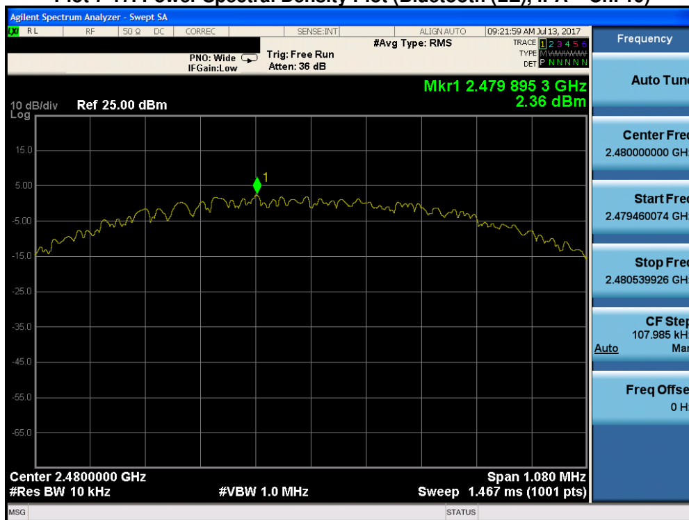
Plot 7-18. Power Spectral Density Plot (Bluetooth (LE), iPA – Ch. 39)
