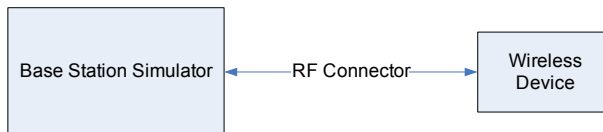
Figure 8-1 Power Measurement Setup
