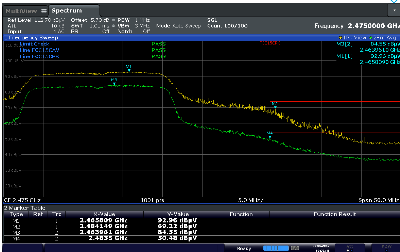
Plot 7-47. Radiated Restricted Upper Band Edge Measurement (Average & Peak)
