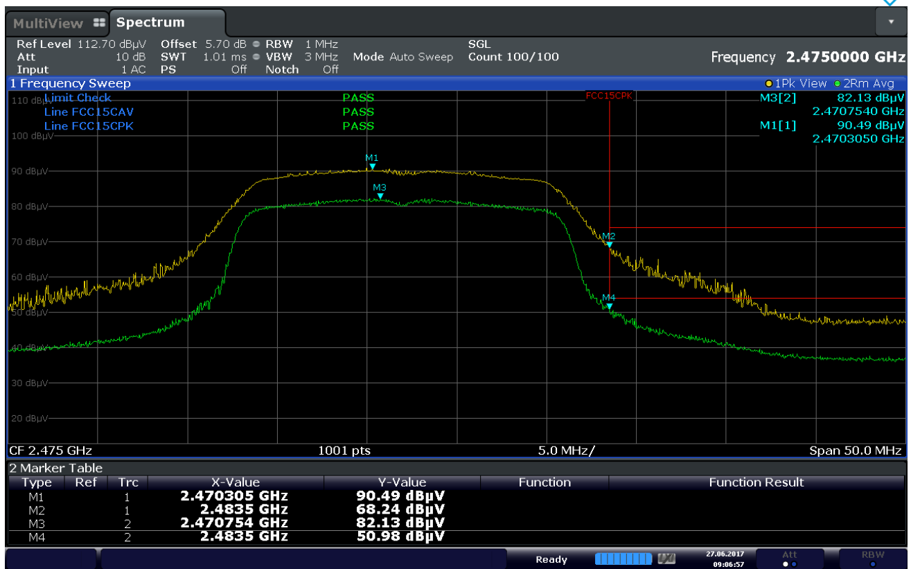
Plot 7-49. Radiated Restricted Upper Band Edge Measurement (Average & Peak)
