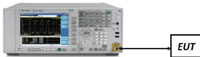
Figure 7-7. Test Instrument & Measurement Setup
