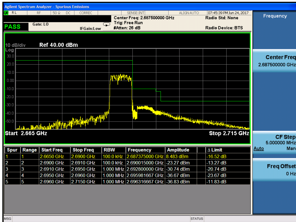
Plot 7-19. Upper ACP Plot (Band 41 – 5.0MHz QPSK – RB Size 25)
