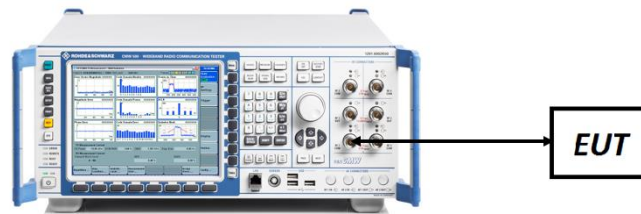
Figure 7-4. EIRP Measurement Setup
