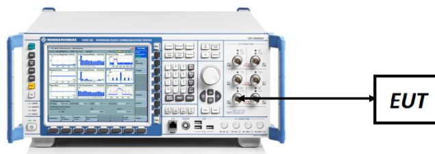
Figure 7-5. ERP/EIRP Measurement Setup
