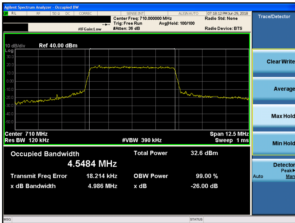
Plot 7-10. Occupied Bandwidth Plot (Band 17 - 5.0MHz 16-QAM - Full RB Configuration)
