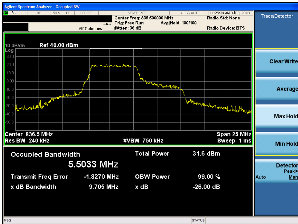
Plot 7-24. Occupied Bandwidth Plot (Band 5 - 10.0MHz 16-QAM - RB Size 27, RB Offset 0 Configuration)
