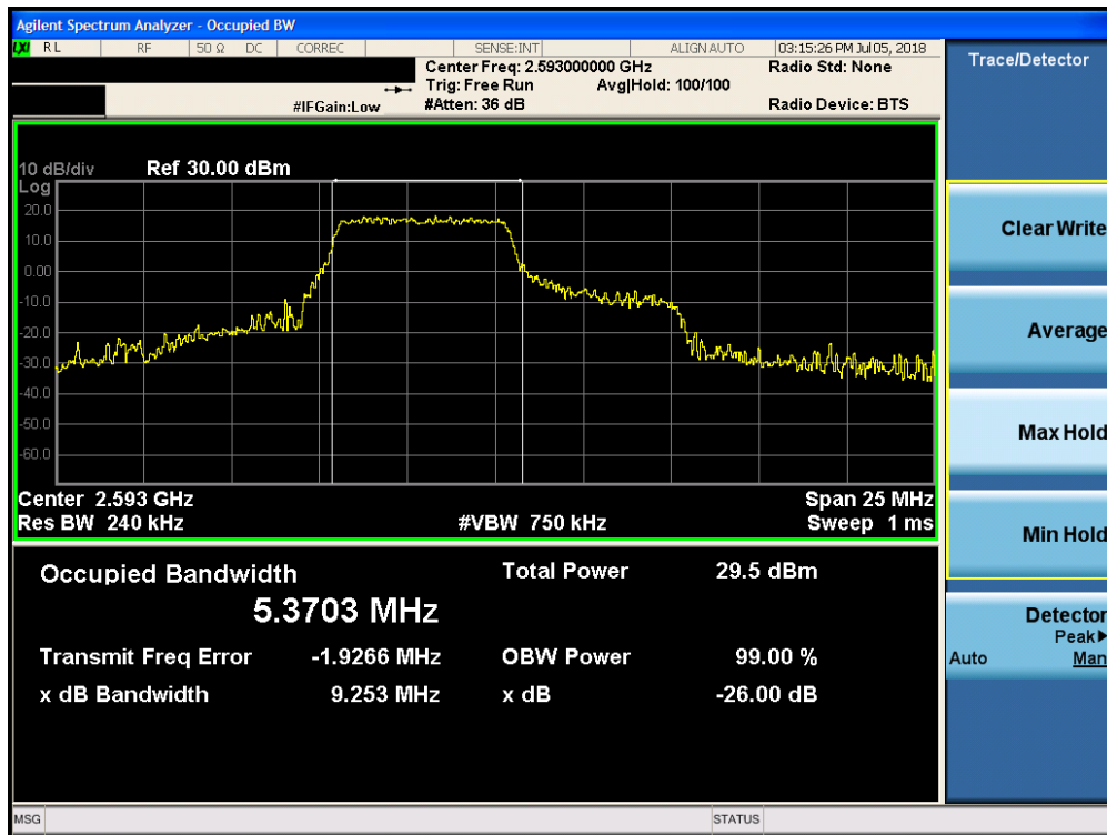
Plot 7-74. Occupied Bandwidth Plot (Band 41 - 10.0MHz 16-QAM - RB Size 27, RB Offset 0 Configuration)
