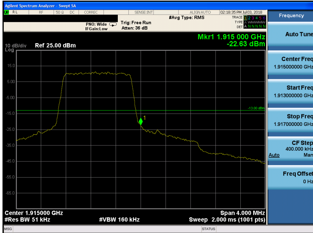
Plot 7-224. Upper Band Edge Plot (Band 25 - 1.4MHz QPSK - Full RB Configuration)
