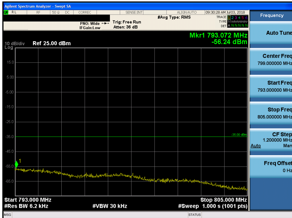
Plot 7-175. Upper Emission Mask Edge Plot (Band 13 - 5.0MHz QPSK - Full RB Configuration)
