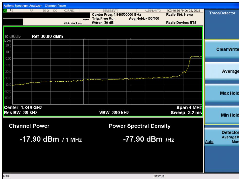
Plot 7-231. Lower Extended Band Edge Plot (Band 25 - 5.0MHz QPSK - Full RB Configuration)
