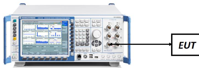
Figure 7-4. Conducted Power Measurement Setup
