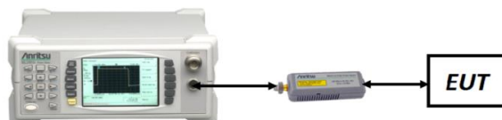
Figure 7-3. Test Instrument & Measurement Setup for Average Power Measurement
