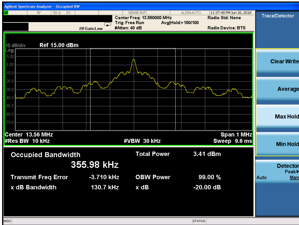
Figure 7-6. 20dB Bandwidth Plot (Reader 100 Ask 1 out of 256)
