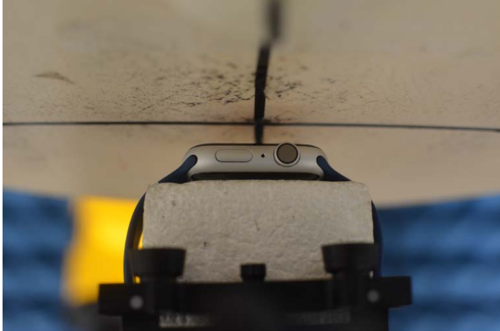
SAR Test Setup Photo 1: Aluminum front side at 1.0 cm with Sport wrist band
