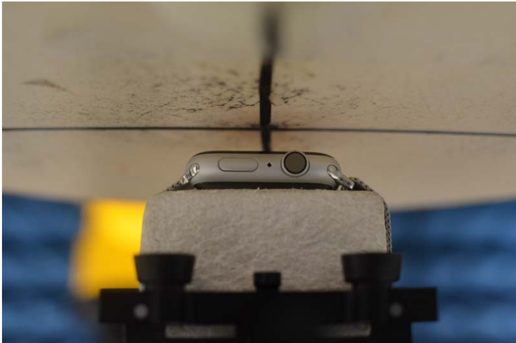
SAR Test Setup Photo 3: Aluminum front side at 1.0 cm with Metal Loop wrist band
