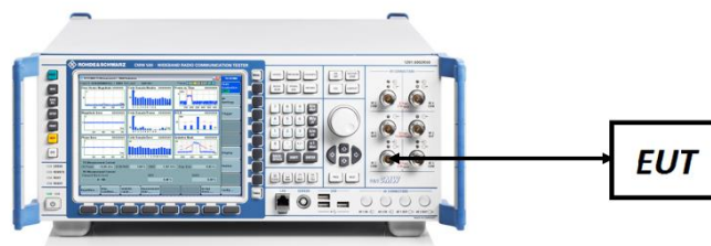
Figure 7-4. ERP/EIRP Measurement Setup
