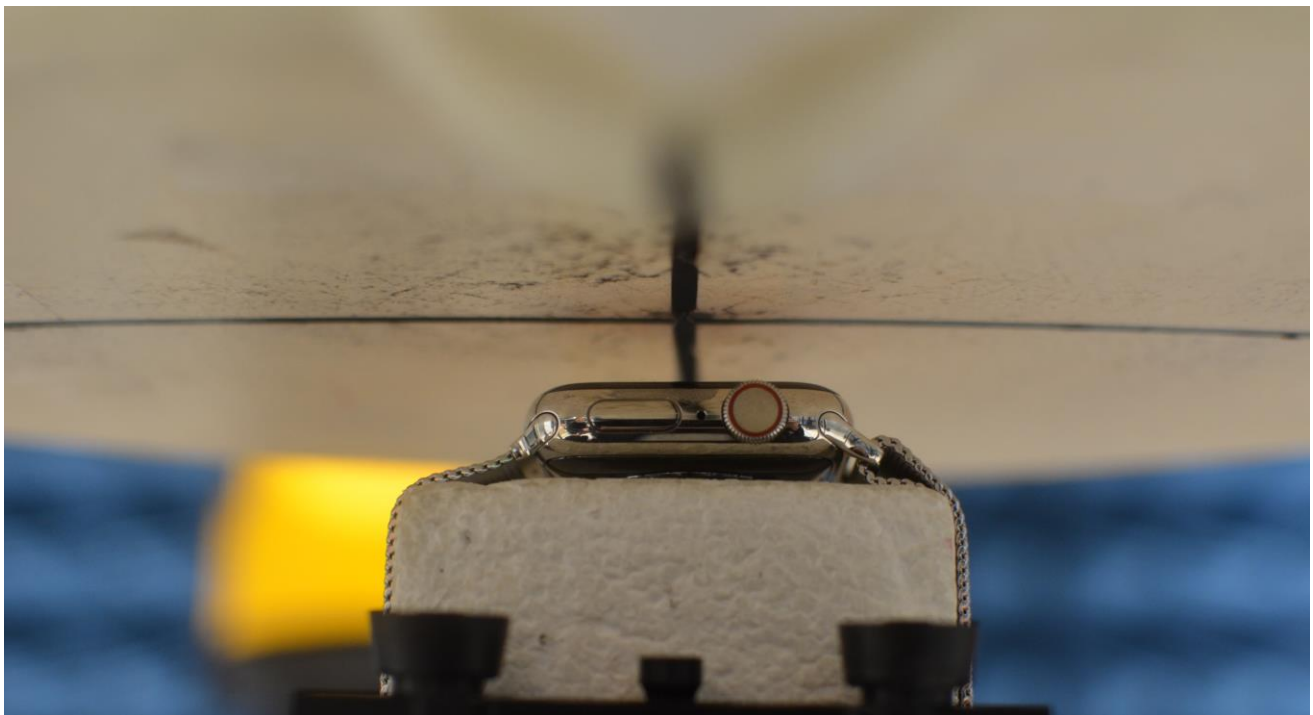
SAR Test Setup Photo 6: Stainless Steel with Metal Loop wristband, Front side at 1.0 cm
