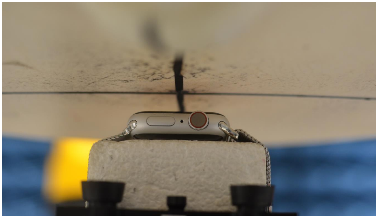
SAR Test Setup Photo 3: Aluminum with Metal Loop wristband, Front side at 1.0 cm
