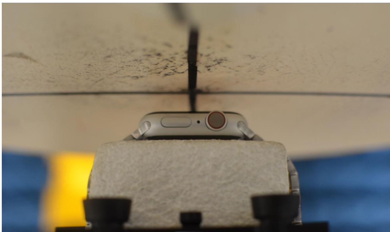
SAR Test Setup Photo 2: Aluminum with Metal Links wristband, Front side at 1.0 cm
