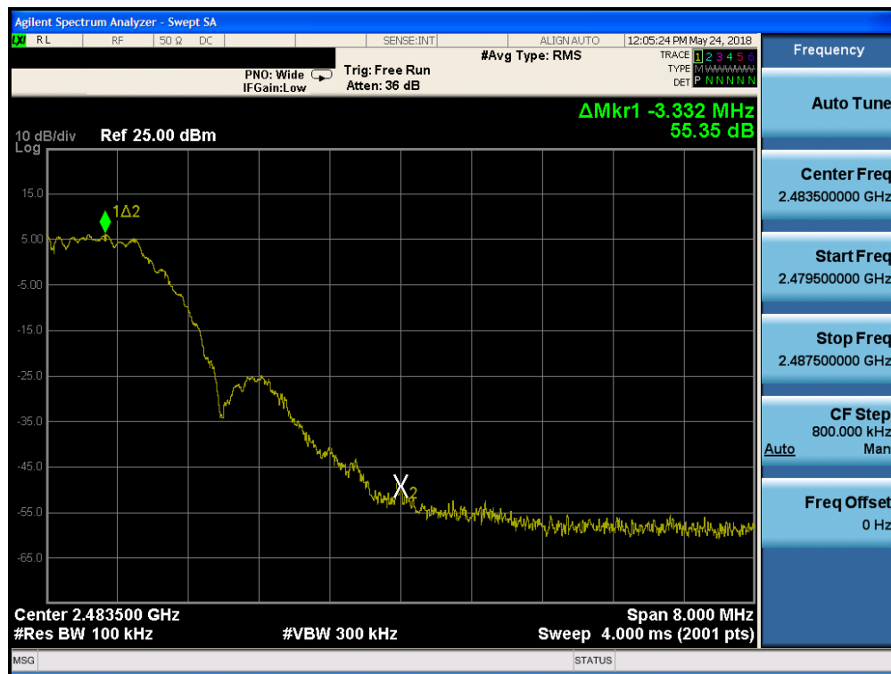
Plot 7-30. Band Edge Plot (Bluetooth (LE), 2Mbps, ePA – Ch. 39)
